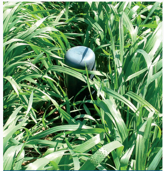
Figure 1: Moisture sensor in wheat crop
